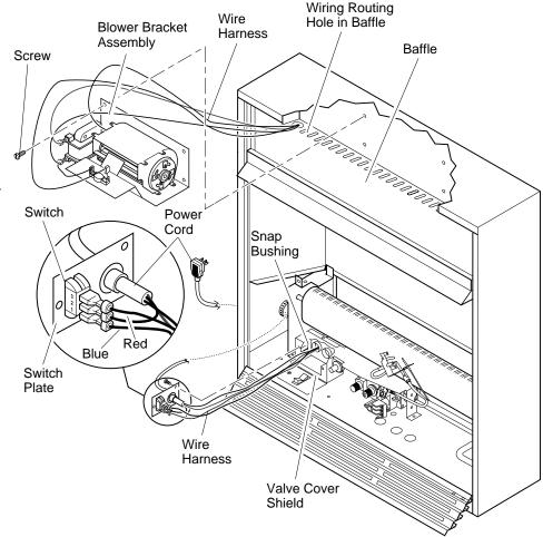
Figure 16 - Installing Blower Bracket Assembly
